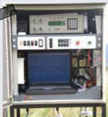
CO 2 , NO x and methane analysers and control PC unit
